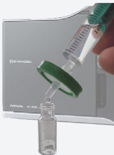
Figure 2: Function and variations of syringe filters
