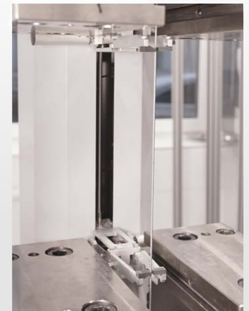
Figure 3: A round steel wire of an ACSR conductor under test
