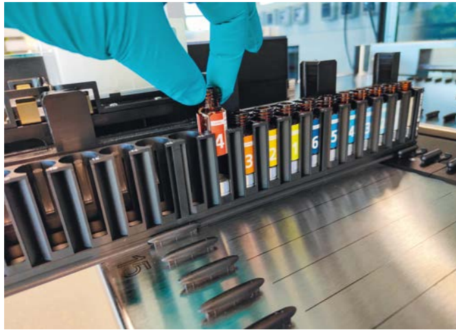
Figure 1: Calibrator and control positioning in robot racks
